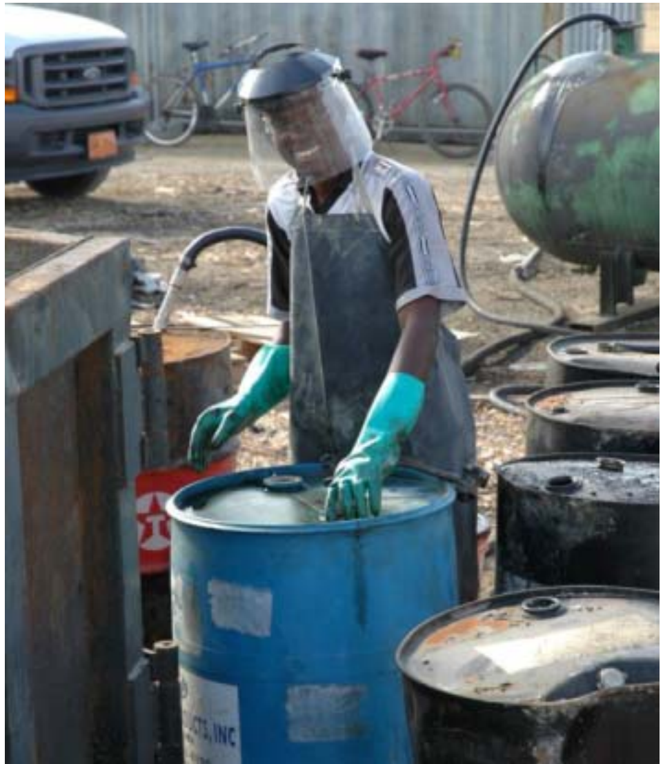
DEH worker, Rohan Lawrence, pumps waste oil from drum into container for further processing.
