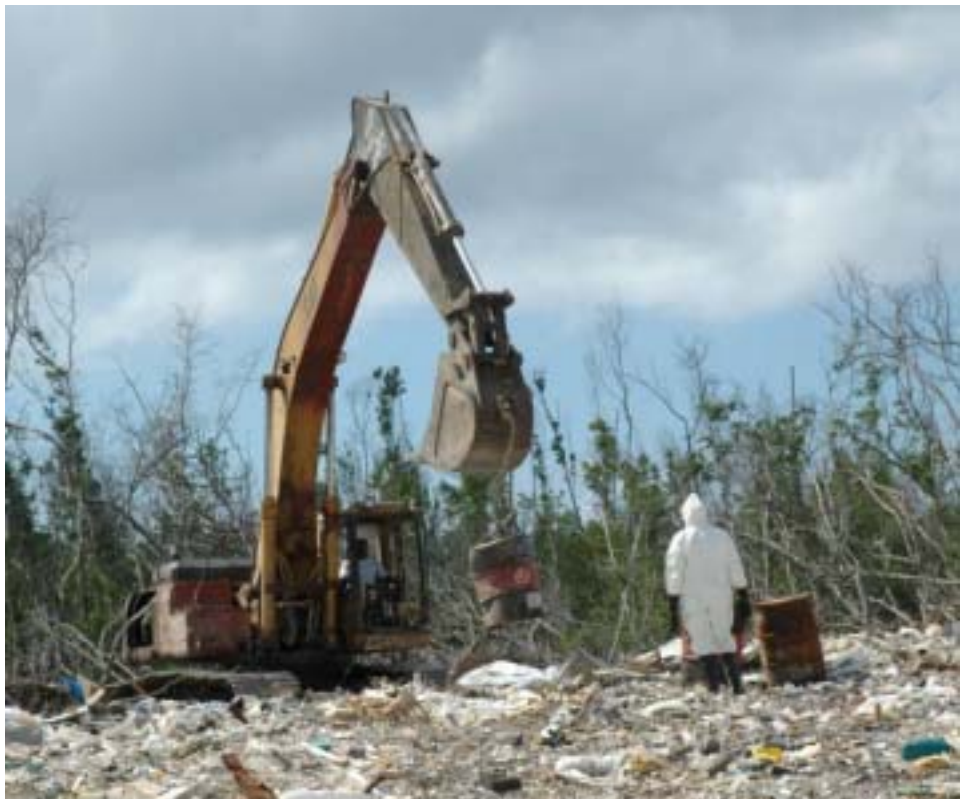
DEH officers use an innovative "sling-method" to safely lift oil drums.
