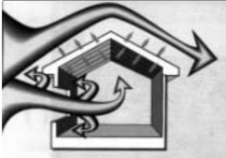
Wind entering your home will demolish the interior and its contents and can cause the roof to blow off.
